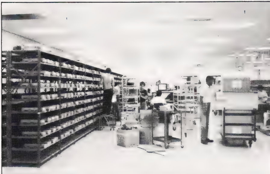
Wall-to-wall Commodore 64s undergoing their 24 hour soak testing. The mobile trolley is connected to each unit in turn.
